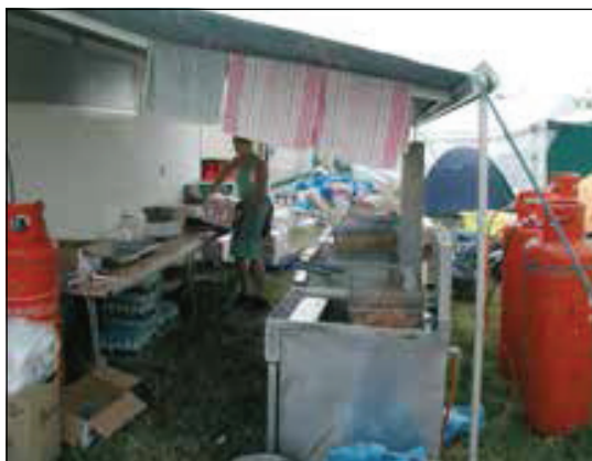
Figure 13: Mobile deep fat fryers too close to combustibles
